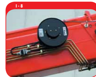
FITTINGS FOR ELECTRICAL SYSTEM FOR ACCESSORIES (*WINCH AND EXTENSION WITH WINCH; *MIXING BUCKET; VIDEO CAMERA)
